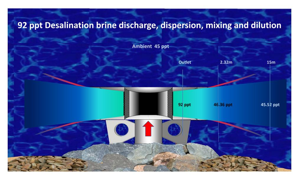
The InvisiHead diffuser discharges effluent in a round surround, up, side ways, straight, and down funneling out flow, and efficiently manages effluent diffusion, dispersion dilution within the near field zone
